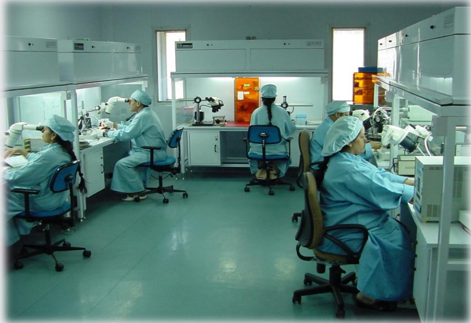
Class 1000 Facility with Work Stations
