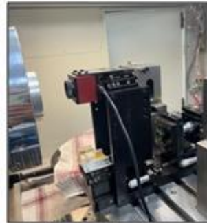
Integration of SHS assembly on CNC Machine
